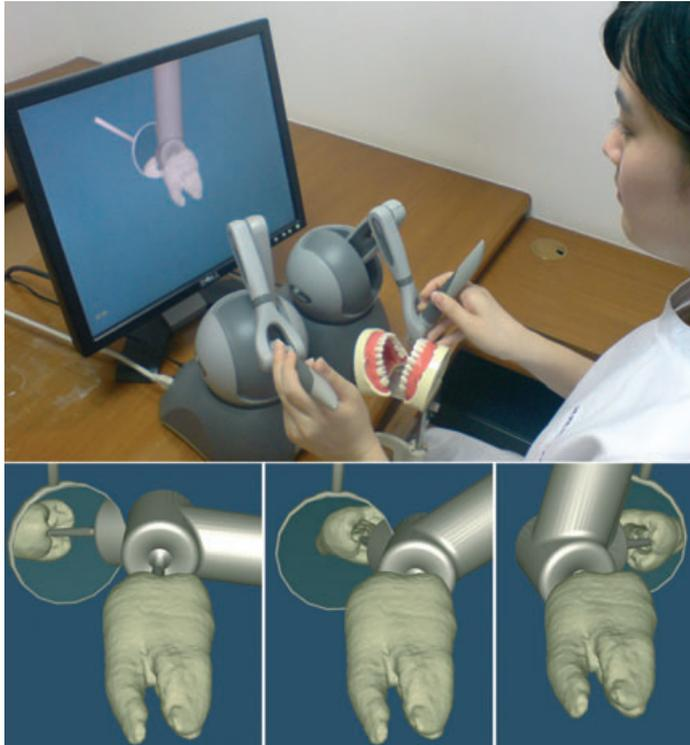
**Figure 2** Three-dimensional models of extracted human teeth were reconstructed from microcomputed tomography images. The virtual reality (VR) simulator was comprised of a 2.8-GHz Pentium 4 PC, with 256 MB RAM and a 13-in computer monitor, connected to two haptic devices.
